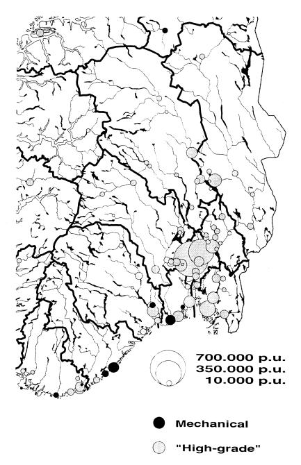
Figure 3. Waste water treatment plants in South-Eastern Norway. Location and capacity of mechanical and "high-grade" plants. Plants with a hydraulic capacity of 5000 p.u. or more in 1991
